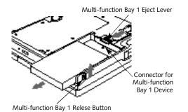
Figure 4-2 Removing and Installing a Device in Multi-function Bay 1
